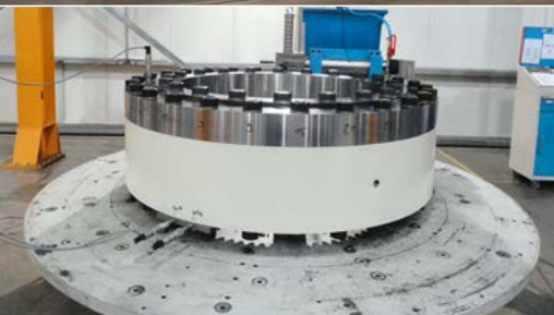
Test rig to verify ▲ bearing seal under pressure
